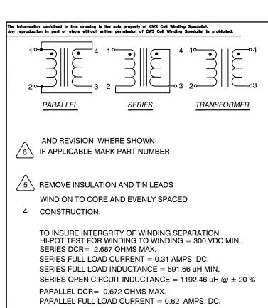
PARALLEL FULL LOAD INDUCTANCE = 147.92 uH MIN. PARALLEL OPEN CIRCUIT INDUCTANCE = 298.12 uH @ ± 20 % SPECIFICATIONS:
